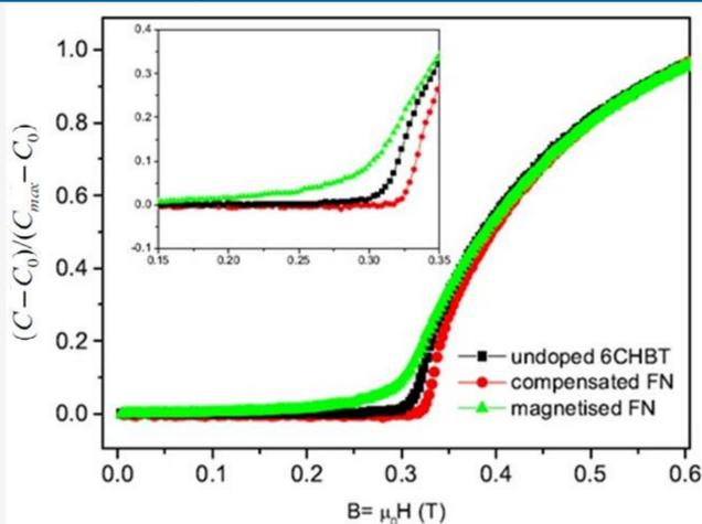
The Fréedericksz transition in the compensated ferronematic occurred in higher magnetic field in comparison with pure nematic while the magnetized ferronematic sample shown well measurable response in capacitance to the applied magnetic field, even much below the Fréedericksz threshold in usual 6CHBT.
