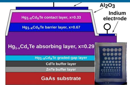
Schematic view of test MIS device based on nBn structure. The inset shows a photograph of the fabricated sample
