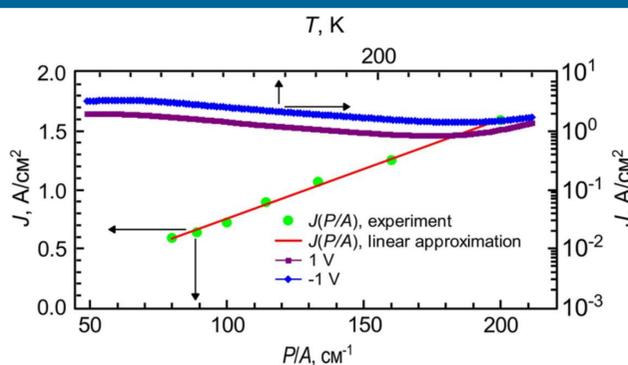
Dependence of the dark current density on temperature and on the ratio of the structure mesa perimeter to area (-2 V, 300 K)
