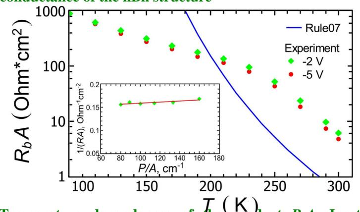
Temperature dependences of the product  $R_b A$ . Inset - dependence of  $1/(R_b A)$  value on the  $P/A$  ratio (2 V, 300 K)
