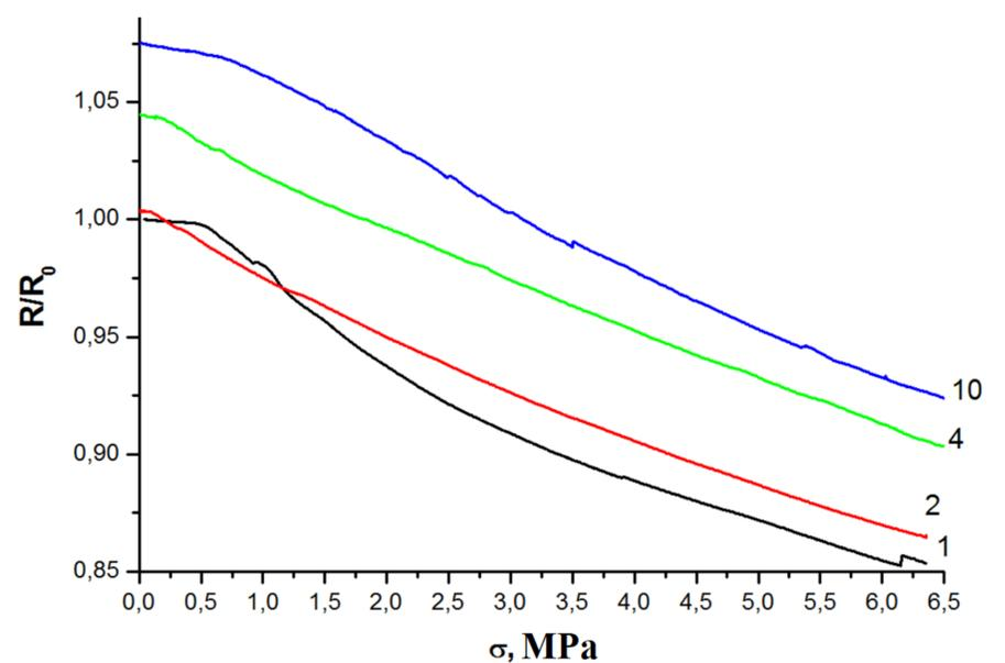
Fig. 1 – Mechanically stimulated change of electrical conductivity of elastically deformed crystals: 1 – first deformation; 2 – second deformation; 4 – fourth deformation; 10 – tenth cycle of elastic deformation.
