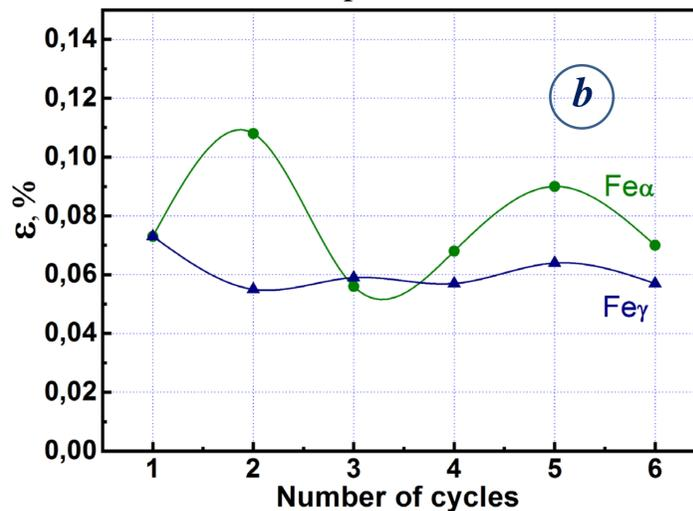
The dependences of the grain size L (a) and the related deformation of the lattice ε (b) of Fe<sub>α</sub> and Fe<sub>γ</sub> phases obtained in NCS layer of 65Г steel from number of cycles of MPT
