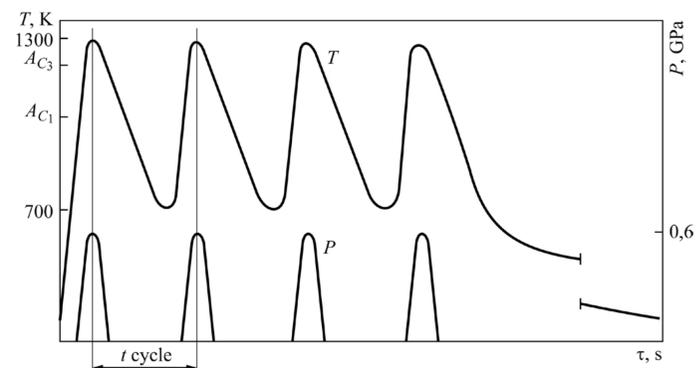
The scheme of cyclic change temperature T and pressure P in the FC zone during MPT
