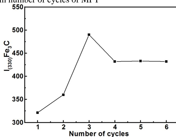
The dependence of the volume fraction of austenite phase in the surface NCS obtained on 65Г steel from number of cycles of MPT      The dependence of the integral intensity I of Fe<sub>3</sub>C peak (330) on X-Ray diffraction patterns obtained on 65Г steel from number of cycles MPT
