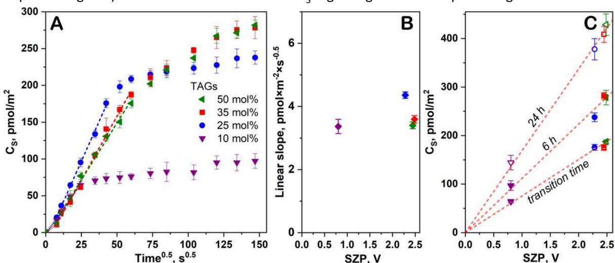
Fig. 1. a) Experimental kinetic curves of AgNPIs deposition on films with different TAG percentage. (b) Impact of film SZP on surface concentration. (c) Experimental and (d) simulated slopes of the linear regime.
