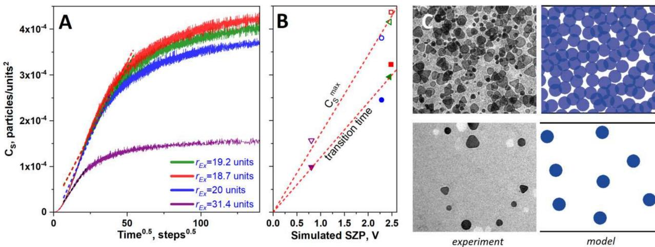
Fig. 2. a) Simulated kinetic curves of disks adsorption on films with different simulated SZP. (b) Impact of simulated SZP on surface concentration. (c) Experimental and simulated arrangement of AgNPIs/disks.
