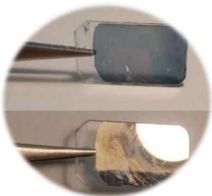
Fig. 3. Appearance of the as-deposited AgNPIs' monolayer in the transmitted and reflected light.
