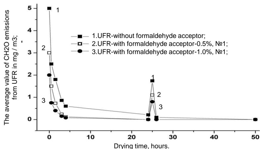
Fig.1. Graphic dependence of gaseous formaldehyde emission, after preparation and drying of component of the developed installatthe use ion. Due to the use of special new chemical gas-forming foamers, the linear and volume shrinkage of UFR was reduced by 3-4 times, to the above values.
