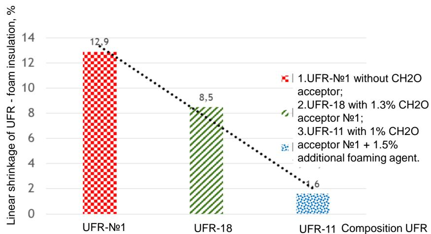
Fig. 2. Dependence of linear shrinkage of industrial foam insulation after production and drying 48 hours, (1-foam insulation without additives KFP-1; 2-foam insulation with the addition of formaldehyde acceptor KFP-18; 3-foam insulation with foamers and acceptor KFP-11.
