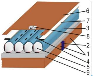
The measurements performed at low frequency by a technique using capacitive coupling of two electrodes with electron subsystem (sketch of cell).
