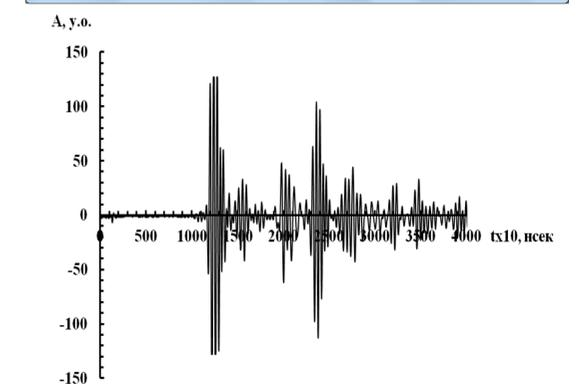
Fig. 7. The illustration of the window for processing data of longitudinal elastic wave velocity measuring  $V_{\parallel} = 2469$  m/sec in nanocomposite polyethylene + 0,7% MWCNT by by impulse-phase ultrasonic method on frequency  $f_{\perp} \approx 1$  MHz.
