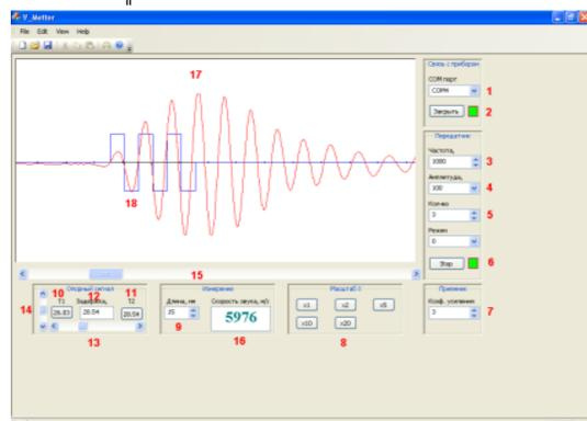
Fig. 3. Illustration of the window for processing data of elastic waves velocity  $V_{\parallel}$  measurements in  $\text{SiO}_2/\text{Si}$  plate by echo-impulse method at frequency  $f_{\parallel} \approx 1$  MHz and the presence of computer device KERN-4
