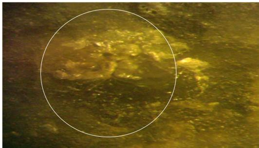
Fig. 2.  $\text{SiO}_2$  surface after the nanosecond laser irradiation by the ruby laser with the intensity of  $I \approx 300$  Mw/cm<sup>2</sup> with the dose  $D = 4 \times 1$  the duration of the ruby laser pulse  $\tau \approx 20$  ns with the wavelength  $\lambda = 694$  nm. The circle indicates the area of the laser irradiation (x56)
