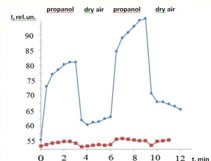
Fig. 8. Relaxation of current in ZnO film when vapor of propanol or dry air is let into the chamber ( $V = 200$  B). Red markers -  $T = 293$  K, blue -  $T = 393$  K.
