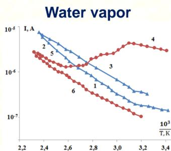
Fig.4. Temperature dependences of current in ZnO film in air atmosphere (1-2-3) and in the presence of water vapor (4-5-6). (V = 200 B)
