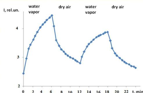
Fig. 6. Relaxation of current in ZnO film at periodic inflow into the chamber of water vapor or dry air ( $V = 200$  B) at  $T = 293$  K.
