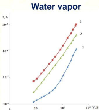
Fig.2. CVC of ZnO film in air atmosphere at 290 K (1) and 420 K (2) and in the presence of water vapor at 290 K (3).
