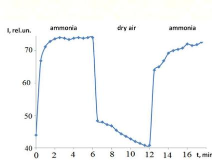
Fig. 7. Relaxation of current in the film ZnO with periodic inflow into the chamber of ammonia vapor or dry air ( $V = 175$  B) at  $T = 293$  K
