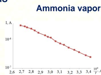
Fig.5. Temperature dependence of current in ZnO film, measured in ammonia vapor (V = 100 B)
