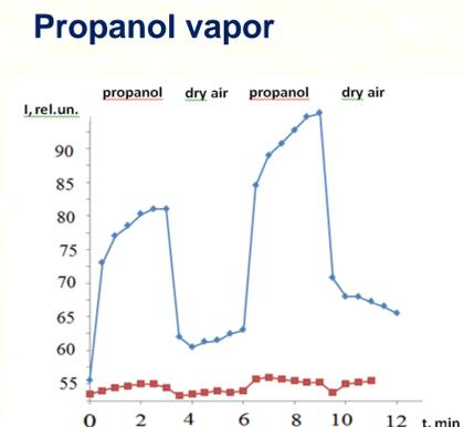
Fig. 8. Relaxation of current in ZnO film when vapor of propanol or dry air is let into the chamber (V = 200 B). Red markers - T = 293 K, blue - T = 393 K.
