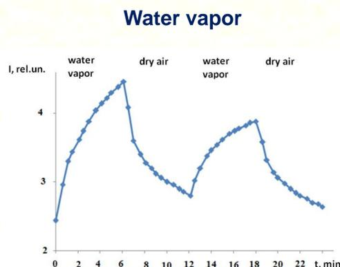
Fig. 6. Relaxation of current in ZnO film at periodic inflow into the chamber of water vapor or dry air (V = 200 B) at T = 293 K.
