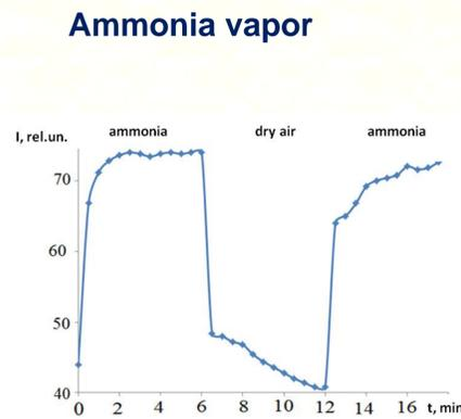
Fig. 7. Relaxation of current in the film ZnO with periodic inflow into the chamber of ammonia vapor or dry air (V = 175B) at T = 293 K
