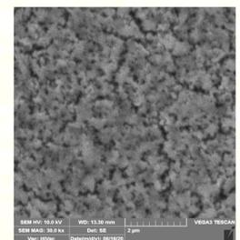
Fig. 1. SEM image of the studied zinc oxide film
