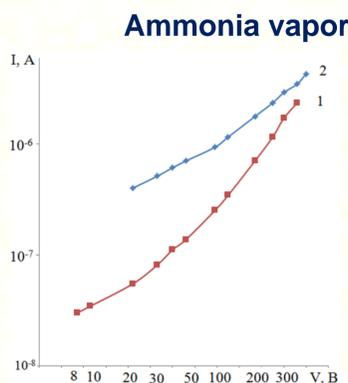
Fig. 3. CVC of ZnO film in air atmosphere (1) and with ammonia vapor (2) at 290 K
