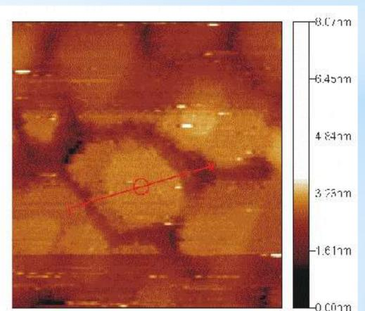
**Fig. 3. Tunnel microscopic images of copper surface on InSe (0001) (JSPM-4610 tunnel microscope).**
