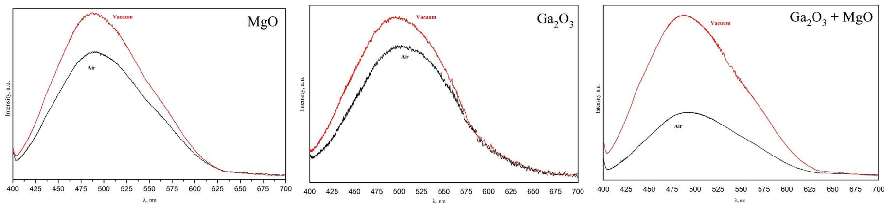
Fig.1. Photoluminescent spectra in air and vacuum (12 Pa) of metal oxide nanopowders
