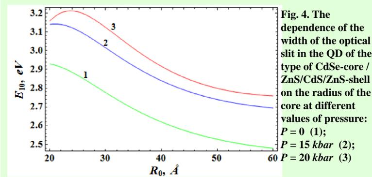
Fig. 4. The dependence of the width of the optical slit in the QD of the type of CdSe-core / ZnS/CdS/ZnS-shell on the radius of the core at different values of pressure:  $P = 0$  (1);  $P = 15 \text{ kbar}$  (2);  $P = 20 \text{ kbar}$  (3)
