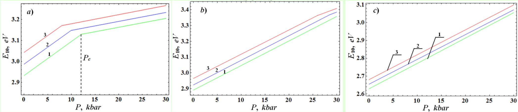
Fig. 3. The dependence of the width of the optical slit on the value of the external pressure in the QD of the type of CdSe / ZnS/CdS/ZnS at different values of the radius of the QD core ( $R_0 = 2 \text{ nm}$  (a);  $R_0 = 2.4 \text{ nm}$  (b);  $R_0 = 4 \text{ nm}$  (c)) and thickness of the shell layers ( $d_2 = a^{(2)}$  (1);  $d_2 = 2 a^{(2)}$  (2);  $d_2 = 4 a^{(2)}$  (3));  $d_i = R_i - R_{i-1}$  is the thickness of the  $i$ -th layer of the shell;  $a^{(i)}$  is the lattice constant
