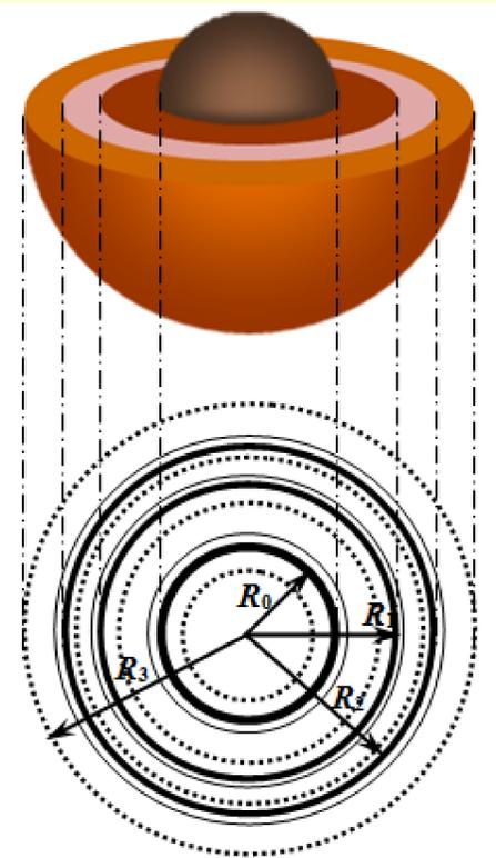
Fig. 1. The geometric model of QD of the type of CdSe-core / ZnS/CdS/ZnS-shell
