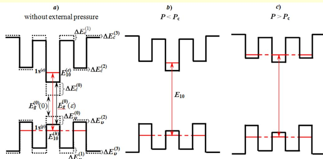
Fig. 2. The zone scheme of QD of the type of CdSe-core / ZnS/CdS/ZnS-shell (solid line) and the zone structure of the corresponding bulk materials (dotted line) in the absence of external pressure (a) and under the action of pressure (b, c)
