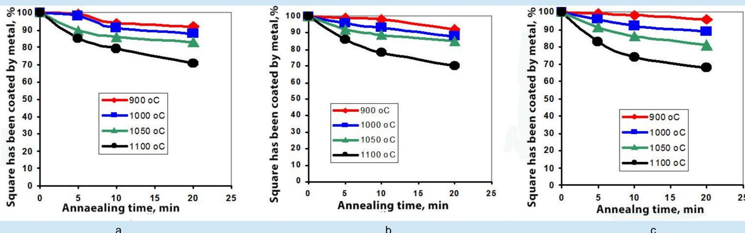
Fig. 2. Dependence of oxide materials area covered by double hafnium-copper film on annealing time at various temperatures (900 - 1100 °C): a – alumina ceramics; b – leucosapphire; c – zirconia ceramics.
