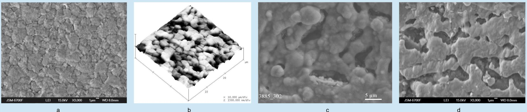
Fig. 1. SEM (a, c, d) and AFM (b) images of double hafnium-copper film deposited onto oxide materials and further annealed at temperature 1100 °C during various time in vacuum: a, b – zirconia ceramics, 5 min; c – alumina ceramics, 20 min; d – leucosapphire, 20 min.
