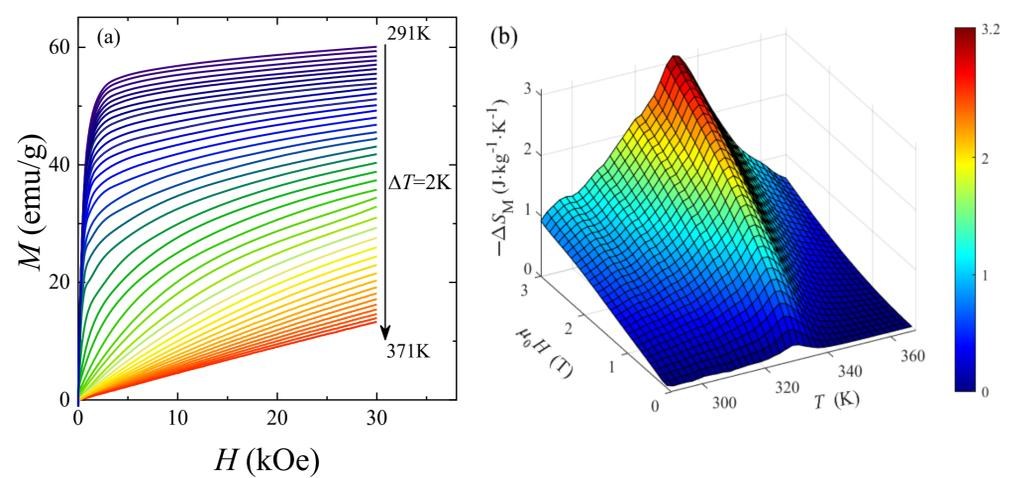
Fig. 3. Isotherms of magnetization within  $T = 291\text{--}371$  K (a), as well as temperature and field 3D-dependence of the magnetic entropy change up to  $\mu_0 H = 3$  T (b) for the selected  $\text{La}_{0.75}\text{K}_{0.2}\text{Mn}_{1.05}\text{O}_3$  nanocrystalline sample.
