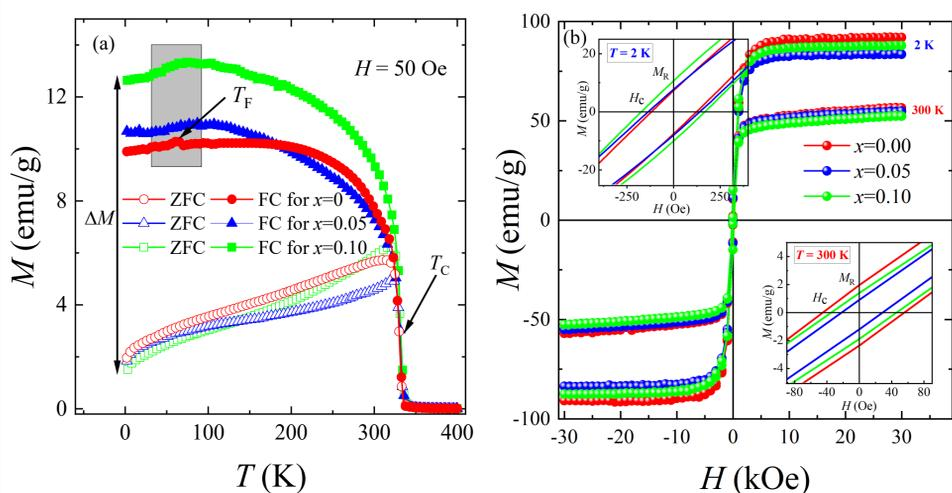
Fig. 2. Temperature (a) and magnetic field (b) dependences of magnetization for the  $\text{La}_{0.8-x}\text{K}_{0.2}\text{Mn}_{1+x}\text{O}_3$  nanopowders. The inserts of (b) show an enlarged area of hysteresis loops at  $T = 2$  and 300 K to determine coercivity  $H_C$  and residual magnetization  $M_R$ .
