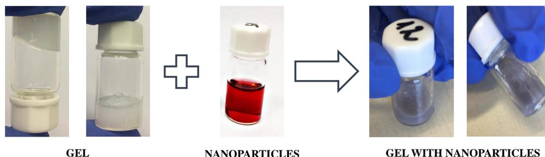
Fig. 3. The process of obtaining supramolecular gel with gold nanoparticles.
