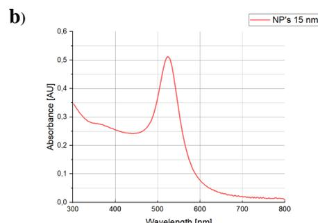
Fig. 2. TEM image (a) and UV-vis absorption spectra (b) of obtained gold nanoparticles.
