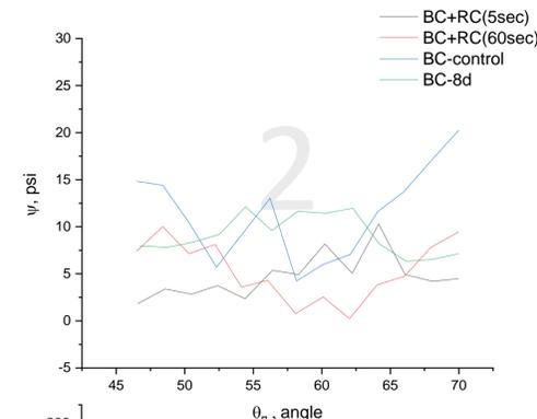
Graphs of the reflection coefficient of the mirror component on the angle of incidence of the laser on the samples obtained from Stokes parameters (1), the dependence of the ellipsometric parameter  $\psi$  (in degrees) on the angle of incidence of the laser on the samples obtained from the Stokes parameters (2) and the ellipsometric parameter  $\Delta$  (in degrees) (3)
