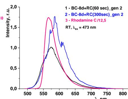
Luminescence spectra of BC-based films GEN-1 (1-4) and GEN-2 (1-2) with Rhodamine C (3); T = 300 K;  $\lambda_{ex} = 473$  nm
