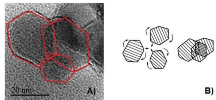
Fig.2. Oriented consolidation (attachment) of ZnO nanoparticles: (A) HRTEM image, calcinations temperature 500 °C, (B) scheme of mechanism.
