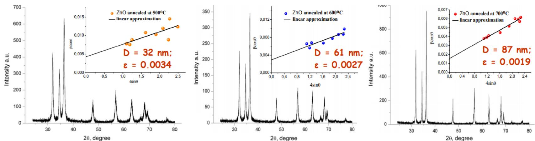
Fig.3. XRD pattern and Williamson-Hall analysis of ZnO nanopowders prepared in agar media prepared
