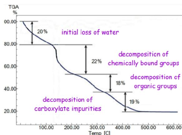
Fig.1. The thermogravimetric curve of the gel.
